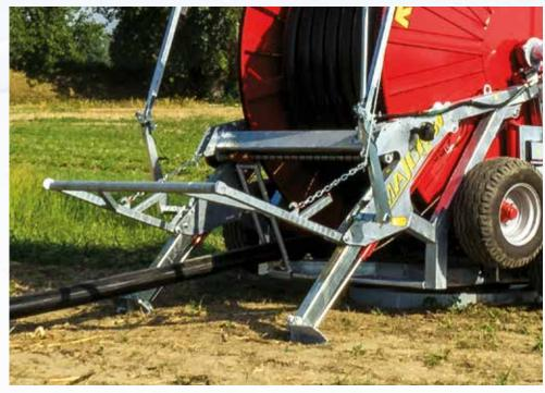
Both the Xj and Xjm range of RM hose-reel irrigation machines feature a structure that can be hydraulically lowered. Therefore, two positions are determined: on wheels to allow its transfer on road or standing on the ground during work phase.
