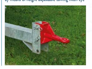
All the XJ and XJM models are fitted with the towing hitch eye whose height can be adjusted through simple gudgeon pins.
