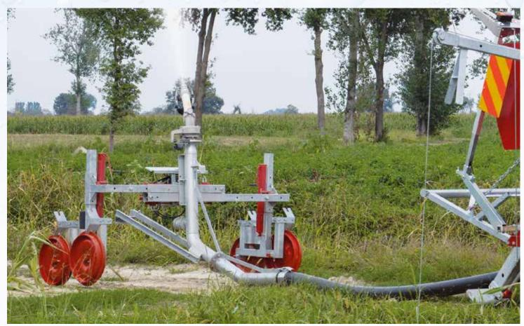
All sprinkler trolleys are available in the two- or four-tyred wheel version or made up of cast iron with directional crests.
