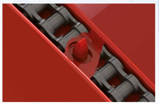
Another remarkable characteristic of RM hose-reel irrigation machines: the **drive between turbo-reducer and reel is manufactured with high-tensile strength** ARNOLD STOLZEMBERG® chain with extruded rollers and without extension.
