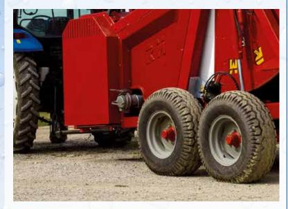
All the machines of the XJ and XJM series fitted with double axle with isodiametric wheels feature the asymmetrical rocker arm.
