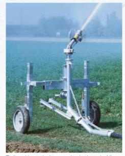
Trolley with standard pneumatic wheels on the XJ model.
