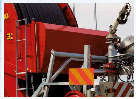
All the XJM models are fitted with a great-capacity fuel tank with a vertical development. This makes it impervious to the machine tilt variations. It is not incorporated into the frame, and it is positioned between diesel engine and reel, or in the rear in the MAGNUM Xim models.
