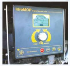
IDROMOP programmer for jointly controllling the irrigation machine + diesel engine on the XJM models.
