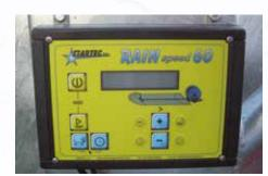
Rain Speed 60 digital metre counter for measuring the rewinding speed.
