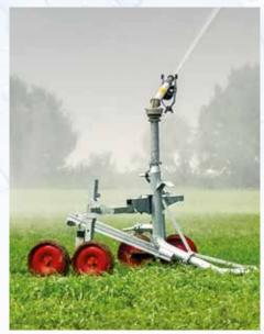
Four-wheel trolley made up of cast iron
