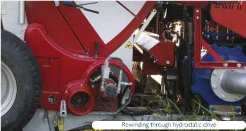
Hose-reel irrigation machines with in-built motor pump are fitted with RM High-Performance Turbo-Reducer to rewind the hose.
