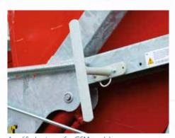
Amplified antenna for GSM module
