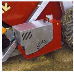
ECU operated by 4-stroke HONDA GX160 engine Hp 5.5 for hydraulic services.
