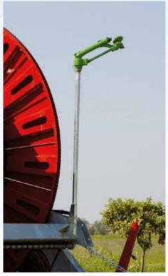
Additional limit switch rain gun controlled by programmer (Skipper or K1 model)  $\,$
