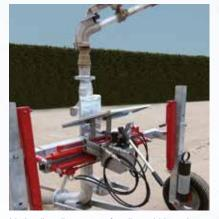
Hydraulic adjustment of trolley width and mechanical adjustment of wheel height
