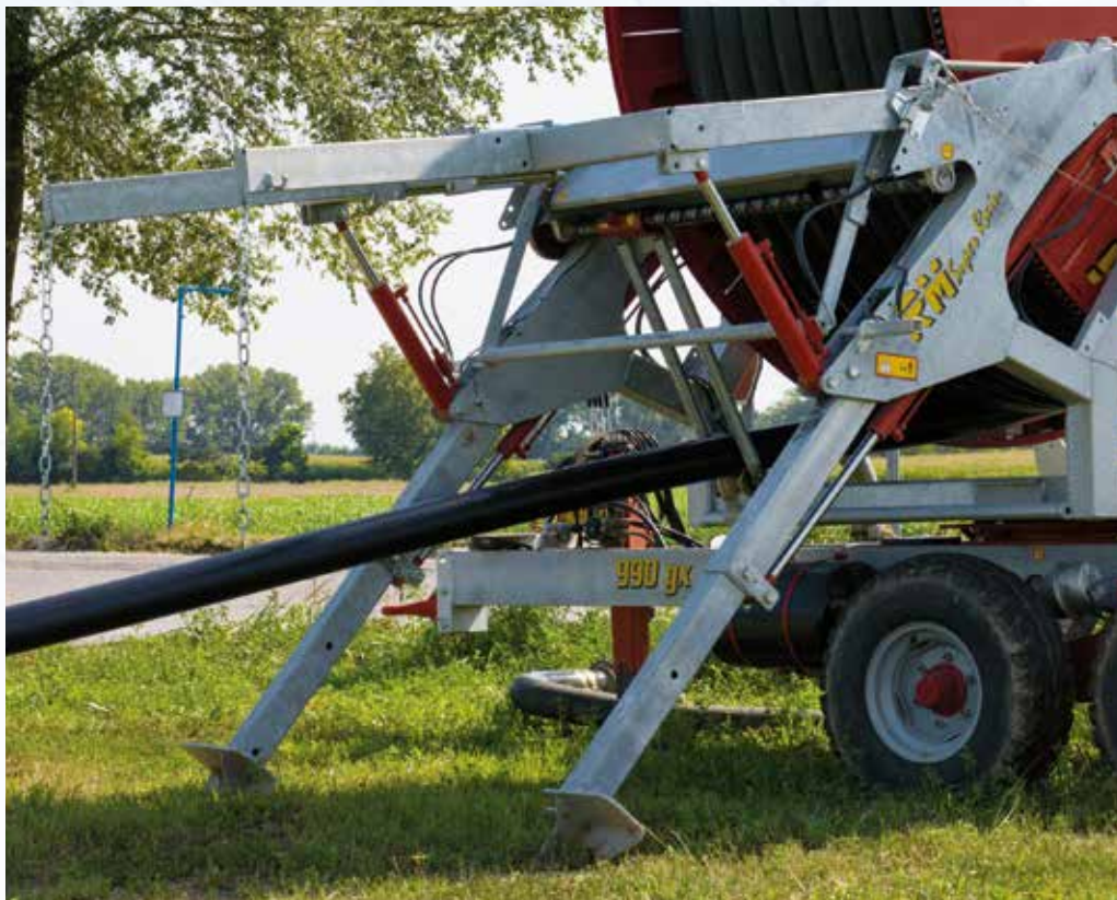
Independent trolley lifting controlled by a couple of hydraulic cylinders (mandatory with spraying boom) for the following models: 581 Gx, 690 Gx, 790 Gx, 890 Gx, 990 Gx e 1100 Gx.
