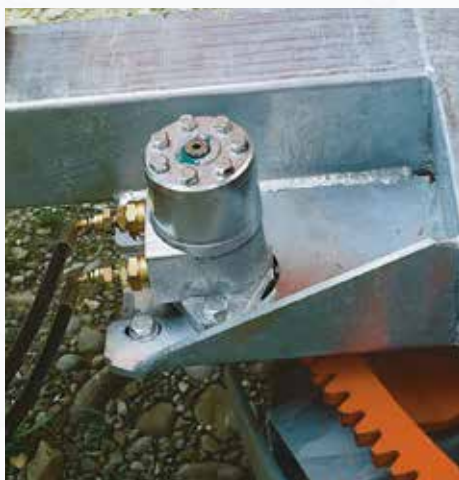
Hydraulic rotation of fifth wheel (standard on all models except for 600 Xj, 700 Xj, 600 Xjm)
