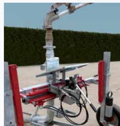
Hydraulic adjustment of trolley width and mechanical adjustment of wheel height
