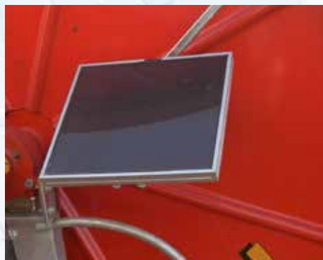
Solar panel for powering electronic equipment.
