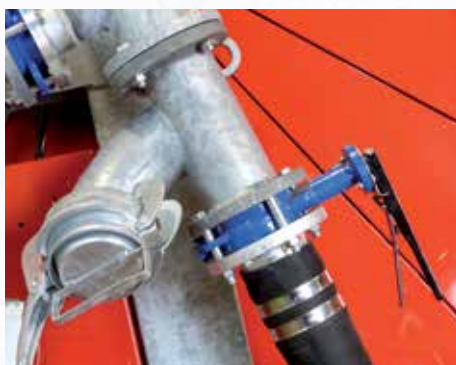
Additional coupler for sludge inlet and turbine cutting off.
