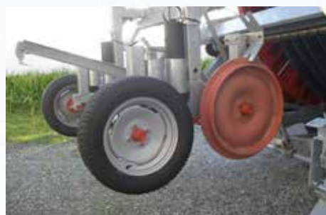
Trolley with two pneumatic wheels and two cast iron wheels
