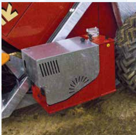
ECU operated by 4-stroke HONDA GX160 engine or by Briggs & Stratton Hp 5.5 for hydraulic services.
