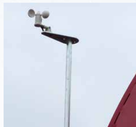
Anemometer for Rain Master 2.6
