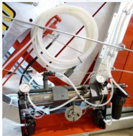
Dosing pump for sewage irrigation with liquid fertiliser.
