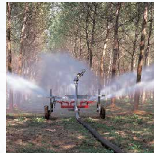
Under-foliage sprinkler device for tall trees
