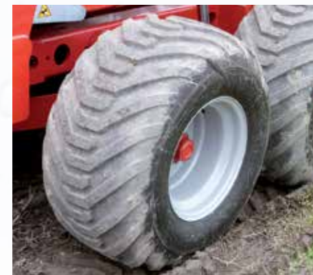
"Big size" type tyre for the Magnum Xj, Magnum Xjm, Magnum Giant models (size 500/50-17)
