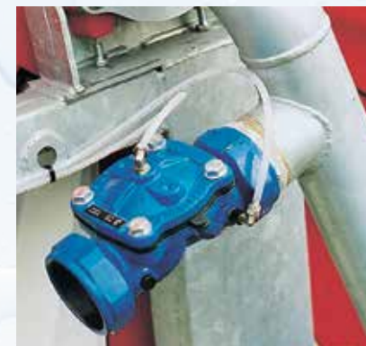
Water pilot operated drain valve.
