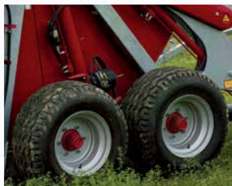
Double axle for asymmetrical compensator (optional for the 800 XJ, 840 XJ, 900 Evo, 800 XJM models)
