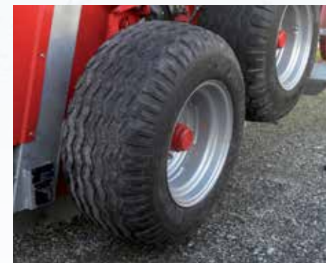
"Big size" type tyre for the 800 jX, 840 Xj, two-axle 900 Evo, 900 Xjm, Major Evo, Major Xjm Evo models (size 15.0/55-17)
