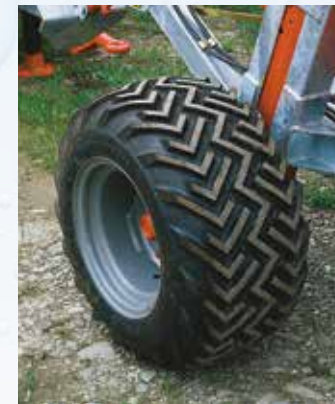
"Big size" type tyre for the 600 Xj, 700 Xj models (size 31x 15.50-15)
