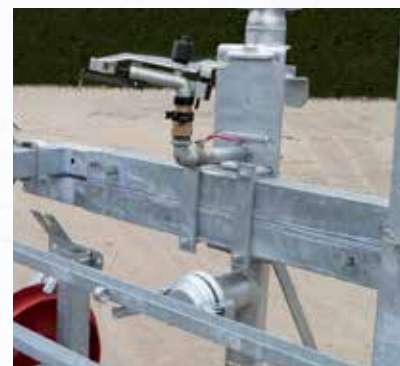
Stretched angle K1 additional rain gun mounted on trolley
